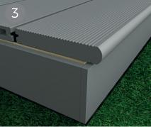
Once the bullnose board has been secured into place you can use a skirting board to neaten the edge. For higher areas you may wish to use a decking board as an edge. Secure the skirting edge with either a screw into each joist or using sumo grip adhesive.
