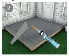
To fit the skirting trim you can either glue this using sumo grip adhesive or the trims can be screwed into the joists (Please note this method may cause the natural fibres to split) We advise the sumo grip adhesive option.
