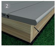
Once the bullnose board is placed you will need to insert a screw at an angle through the supporting joist underneath the board. Ensure the bullnose board is supported along the length with joists and a screw is inserted into each one.
