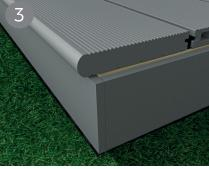
Once installed, you can then cut and place the second piece of trim along the edge until you have the desired finished look. A **gap of at least 8mm** should be maintained between skirting trims and the ends and sides of boards.
