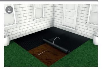
Remove the turf until the ground is completely even. Cover the area of your site with a layer of weed control fabric to prevent any weed regrowth coming up under your decking. You may need to cut the weed mat to fit. You may want to pin your weed mat down at this stage.
