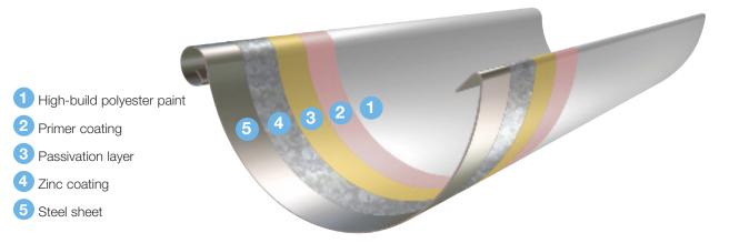
An extra-durable high-build polyester paint coating provides protection and extends the life expectancy of Rainline in excess of 70 years with minimal maintenance, only annual cleaning is recommended and touch up of any scratched paint.
