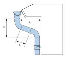
The measurement U is the projection of the offset. An SOKN one-piece offset is available with a fixed projection of 100mm.
